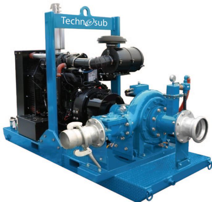
Technosub® Standard High Head Auto Prime pumps are specifically designed to effectively handle a wide range of liquids in applications such as liquid transfer, wash down, fire protection, fracking and jetting where high heads and pressure are required.
