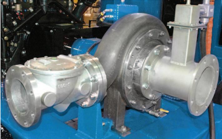
Pump wet end components made in CD4MCu offer superior corrosion resistance, hardness, and impact properties that make the alloy highly abrasion resistant in applications where pumps are subject to abrasive wear and chemical corrosion.
