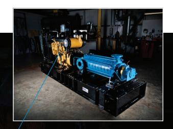
Technojet MH pump driven by **ELECTRIC MOTOR** or **DIESEL ENGINE** standardized with a flexible coupling.
