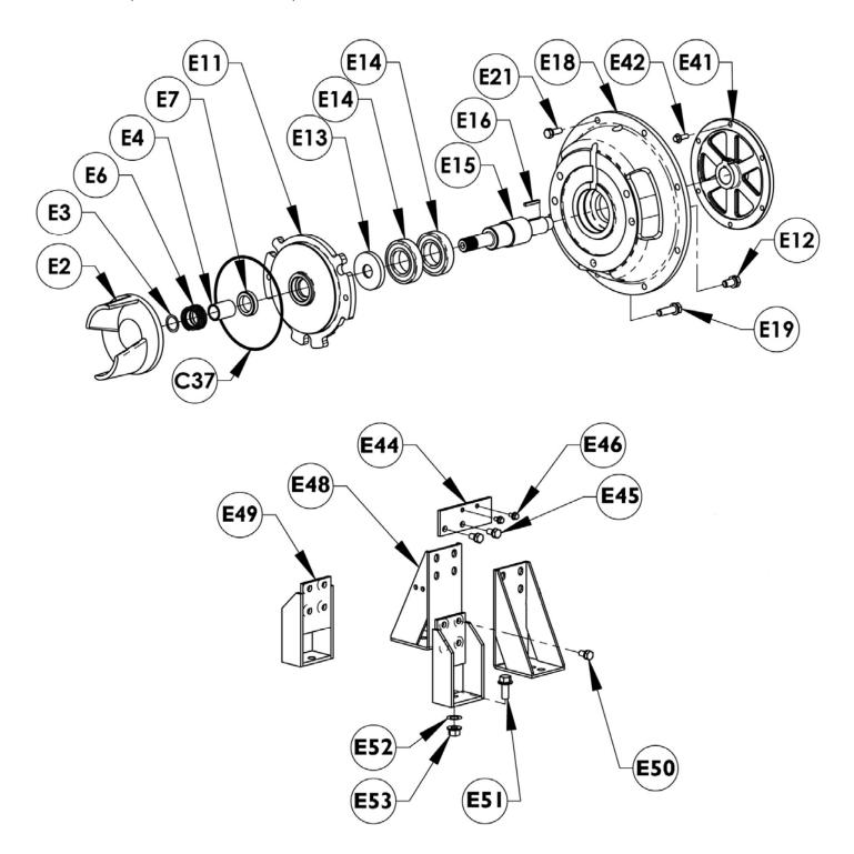
**Repair Parts List - Engine Explosion**
