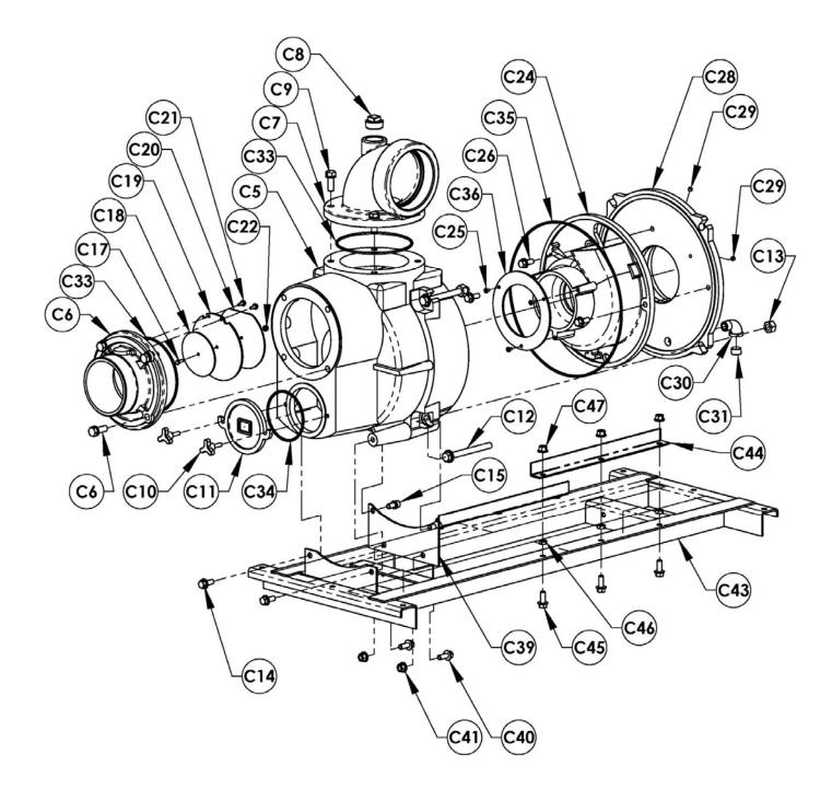
**Repair Parts List - Casing Mounting Explosion**
